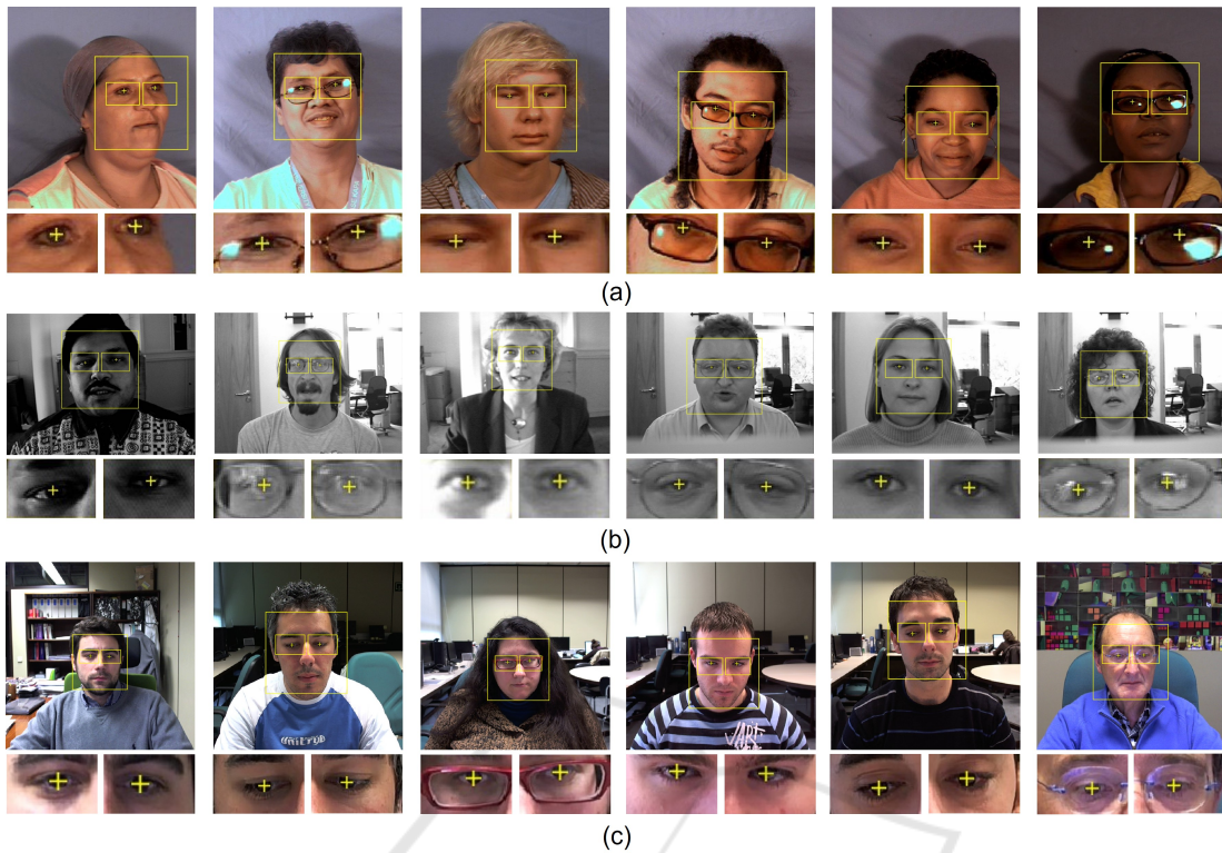
Figure 3: Precise eye center localization results on MUCT (a), BioID (b) and Gi4E (c) databases.
