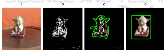
Figure 1: GrabCut pipeline showing the input image (a), the background filter found (b), the most important contour found (c), and the final result (d).
