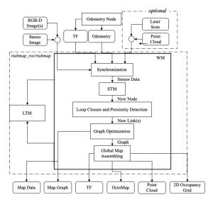
Figure 3: RTAB-Map main node schematic.
