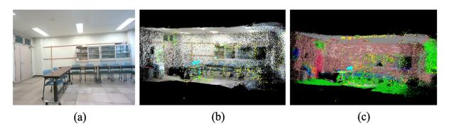
Figure 9: (a) Movement ascertainment environment, (b) pre-existent RTAB-Map output, (c) output of RTAB-Map labeled with a semantic segmentation output image.
