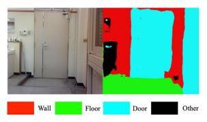
Figure 1: Identifying a floor with a step as a continuous single-level domain.
