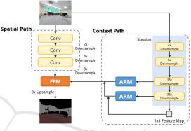
Figure 4: BiSeNet schematic.
