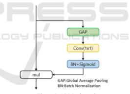
Figure 5: ARM schematic.
