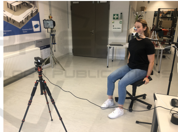
Figure 5: Setup of the experiment. The subject sits at a defined distance in front of the depth camera and breathes through a spirometer attached to a microphone stand. The nose is closed with a nose clip.
