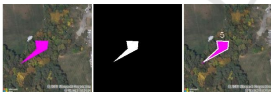
Figure 8: Polygon extraction using an edge detection technique. The generation of a binary mask allows to extract the polygonal coordinates of the designated fire region.
