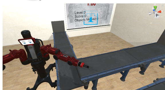
Figure 9: Conveyor belt that delivers the objects to Baxter.
