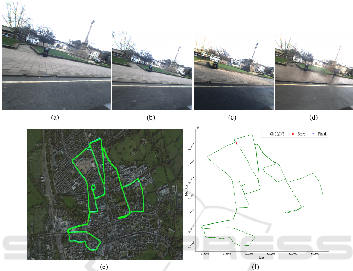
Figure 1: Examples from the Oxford Radard RobotCar outdoor dataset. Top: Images from the same location in the three selected test sequences: a) Gallery: cloudy b) Test 01: cloudy c) Test 02: sunny d) Test 03: rainy (Grasshopper2 left monocular camera). Bottom: 19 km route of the test sequences, e) satellite view f) GNSS/INS.
