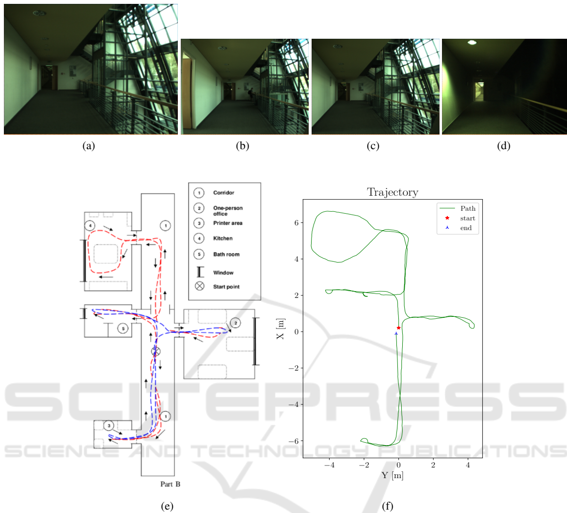
Figure 2: Examples of COLDF indoor database (Pronobis and Caputo, 2009). Images of same location in different sequences: a) Gallery: Cloudy-seq1 b) Test 01: Sunny-seq1 , c) Test 02: Cloudy-seq2 , d) Test 03: Night-seq3 , e) Map view of the lab: blue dashes: standard path consisting of rooms in most typical office environments, red dashes: extended path containing rooms specific to this environment or its part, arrows: direction of driving the robot and f) Robot path of approximately 50 m.
