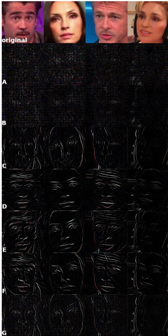
Figure 1: Results of applying SRM filters. The series of photos marked with letters represent: A) 5 \times 5 mask B) a vertical directional mask C) left diagonal directional mask D) horizontal directional mask E) right diagonal directional mask F) 3 \times 3 mask G) combination of 5 \times 5 masks, 3 \times 3 and the horizontal directional for the grayscale image. A constant value enhanced the obtained images for better visualization.
