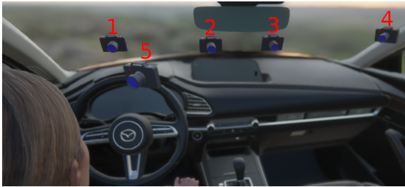
Figure 6: Visualization of all the camera positions of all the synthetic experiments. Camera 1 represents the first camera used for all experiment setups. For the second camera, the specific location changes: Camera 2 is used for the camera pose with label Side , camera 3 for Far Side , camera 4 for Regular , and camera 5 for Near in Table 2.
