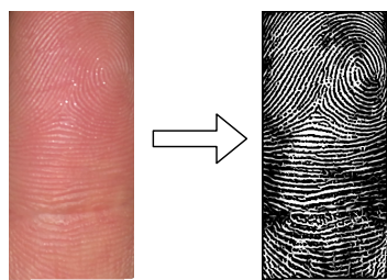
Figure 1: Illustration showing conversion of Finger-Photo to Fingerprint like pattern using Frangi (Frangi et al., 1998) used by Wasnik et al. (Wasnik et al., 2018).
