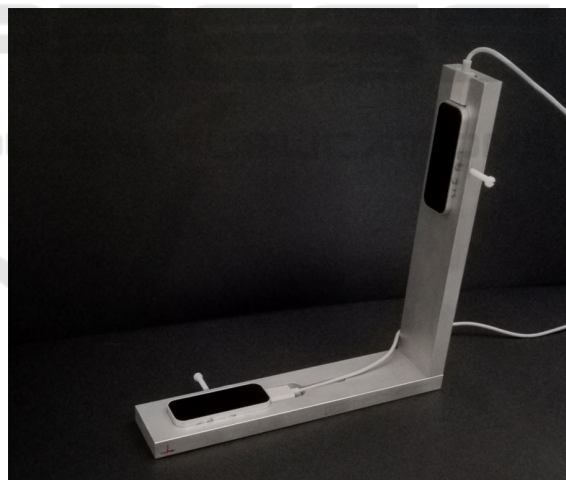
Figure 1: Orthogonal LEAP sensors assembly in VG.
