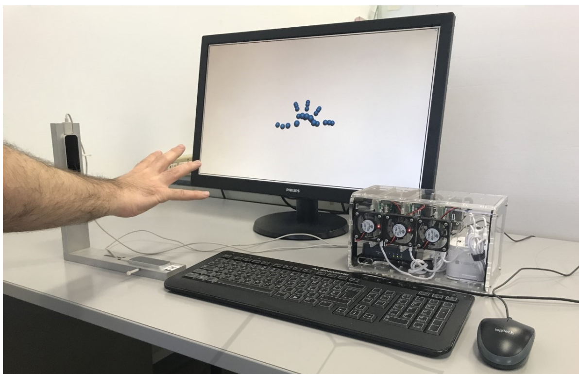
Figure 4: RPi-based VG in its final embodiment, composed by: RPi-box (lateral view, the cooling system is now visible), sensor support, wide-screen, keyboard and mouse.
