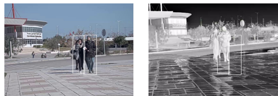
Figure 6: Illustration of the misalignment problem between thermal and visible cameras of the robot.
