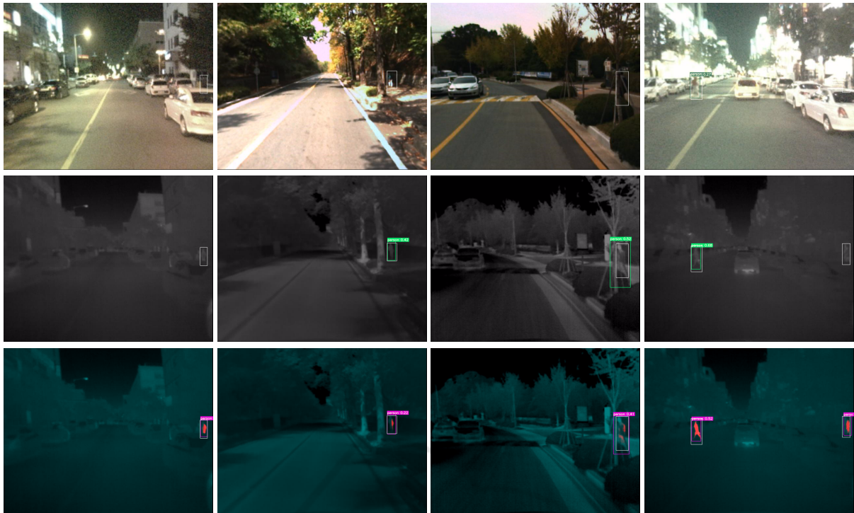
Figure 4: Qualitative results of our proposed method on four sample images from KAIST. From top to bottom rows, visible images with their corresponding thermal images and the resulting saliency maps are shown. For each sample image, the detection results are shown in different color and the corresponding annotated bounding boxes in white color.
