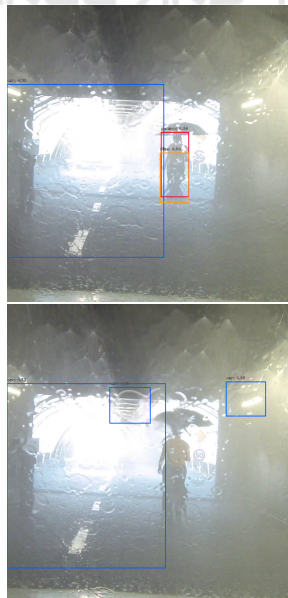
Figure 4: Examples of false positives detection in adverse weather conditions. Blue red and orange bounding boxes respectively denotes car, person and bike detection.
