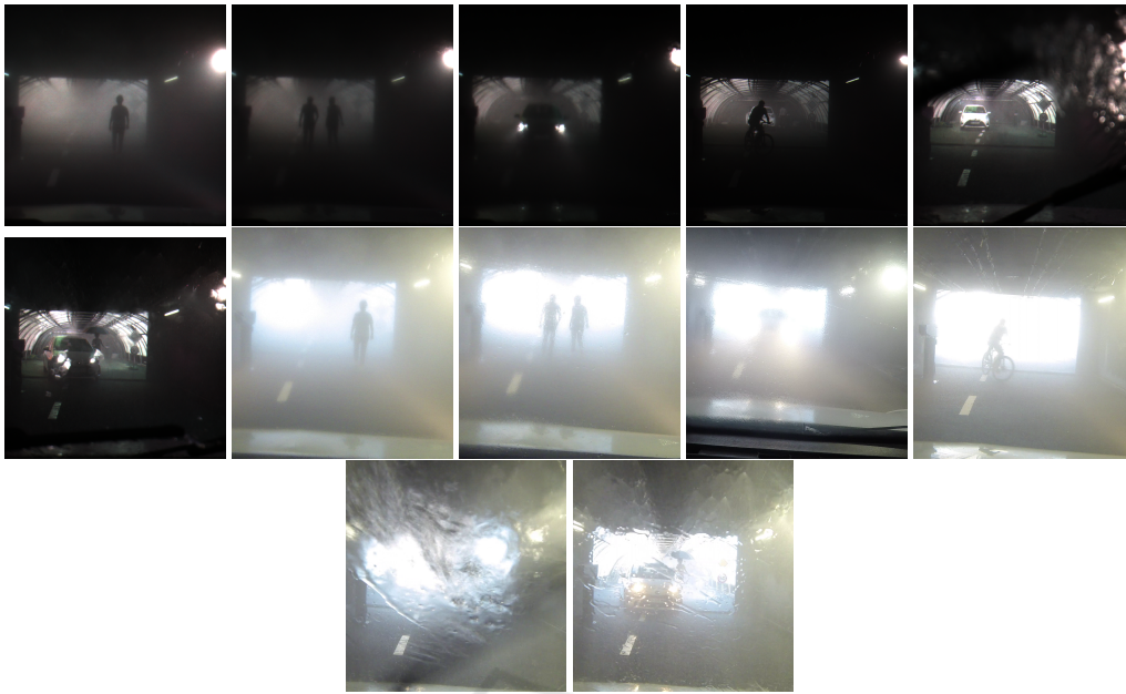
Figure 2: Example of acquisitions at the CEREMA tunnel. The first row are the polarimetric intensity images I = (I_0, I_{45}, I_{90}) and the second row is their equivalent in RGB.
