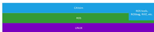
Figure 14: CAVPsim on top of ROS which also uses some general ROS tools.
