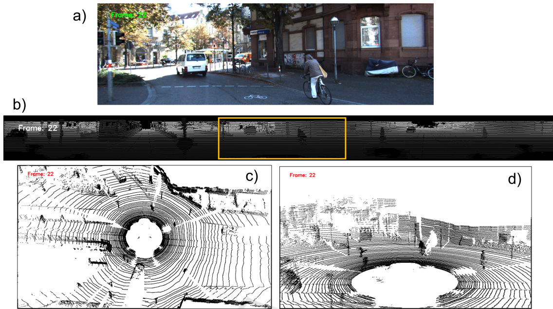
Figure 7: LiDAR data from the KITTI dataset: a) Original image from a color camera mounted on the vehicle, b) 360 degrees LiDAR data, the yellow rectangle corresponds to the color camera field of view, c) Top view of point cloud in 3D, d) Bird's eye 3D view of point cloud.
