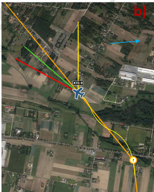
Figure 9: An example of a UAV flight simulation on a route segment, when the maximum roll angle of the UAV has been defined.
