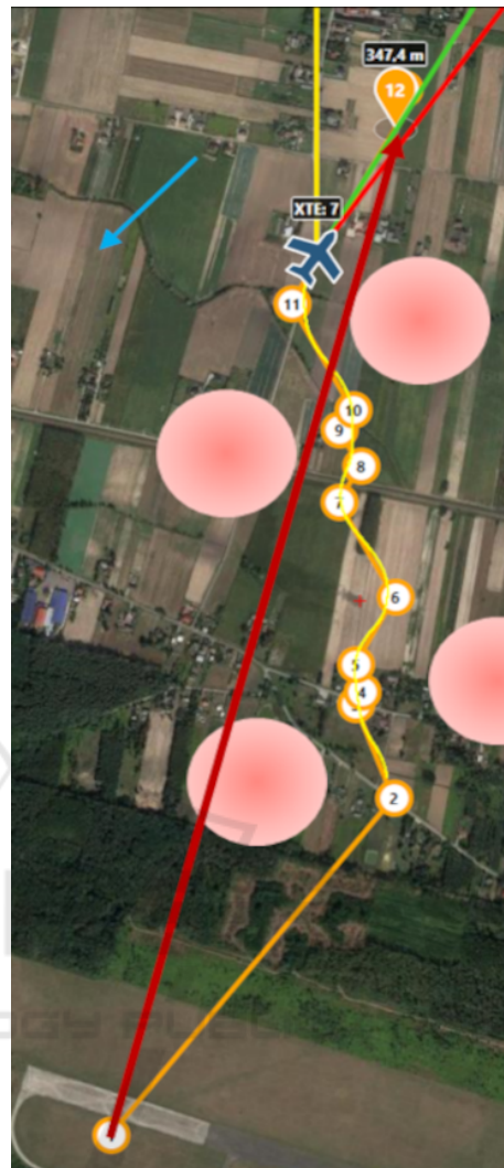
Figure 7: Simulated UAV trajectory for predefined wind speed and direction.
