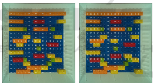
Figure 9: Left Image: grid calibrated with respect to the bricks (on the left) and to the plate (on the right).
