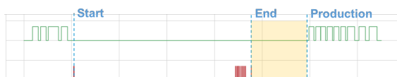
Figure 6: Definition of cluster duration. The faded orange box indicates the uncertainty generated by the process.
