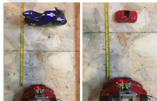
Figure 4: Example of measures performed by sensor and verified by the use of a rule in order to compute the precision.
