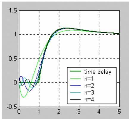
Figure 8: Plant  $G(s) = e^{-\tau s} \frac{K}{T_1 s + 1} \left( 1 + \frac{T_d s}{Ts + 1} \right)$ ,
