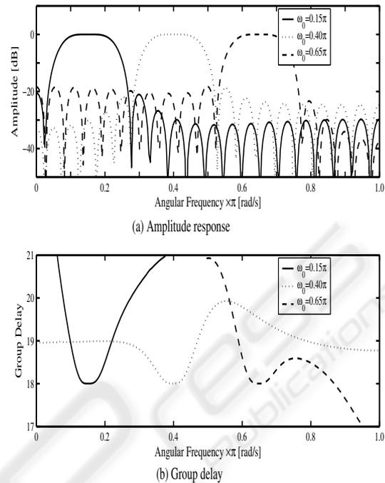
Figure 6: The amplitude response and the group delay response of the bandpass filters for some center frequencies
