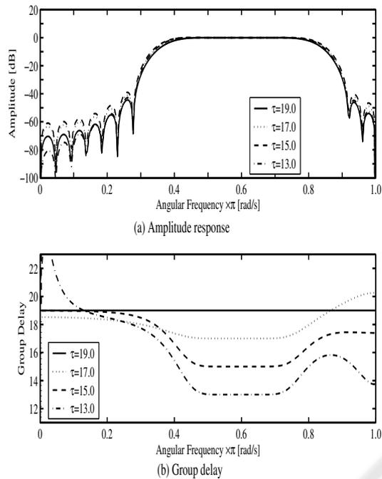
Figure 5: The amplitude response and the group delay of filter of case 4
