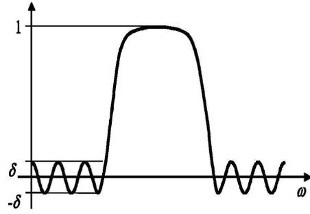
Figure 1: Amplitude response of  $|U(e^{j\omega})|^2 \tilde{V}(e^{j\omega})$
