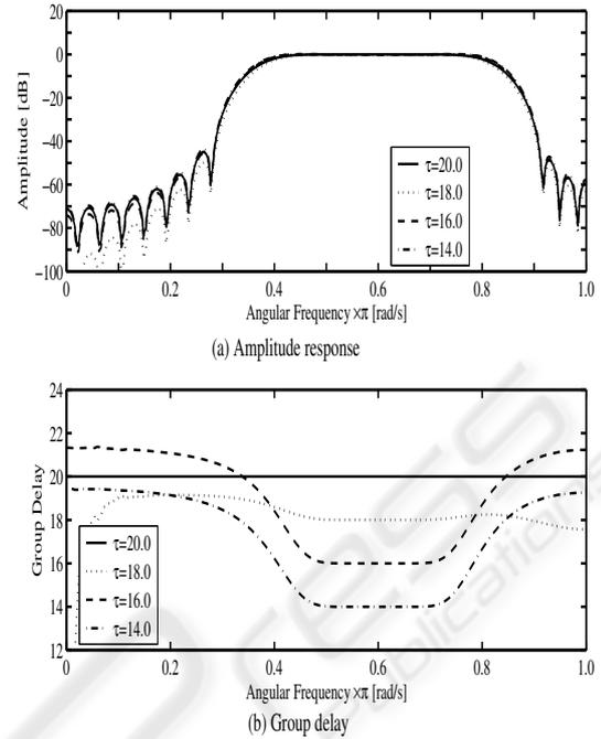
Figure 2: The amplitude response and the group delay of filter of case 1
