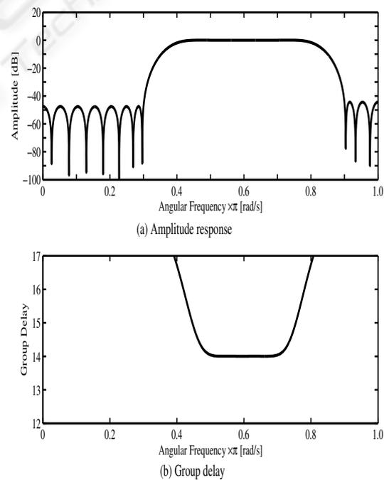
Figure 7: The amplitude response and the group delay response of the bandpass filter with equiripple characteristics in the stopband
