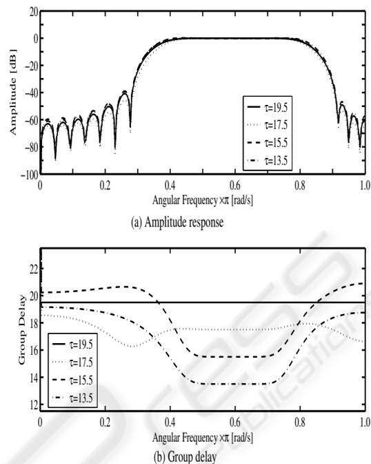
Figure 4: The amplitude response and the group delay of filter of case 3
