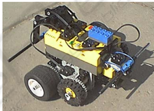
Figure 2: Lego Mindstorms robot. Light sensor is at the top in the front, directed forwards. One touch sensor is installed at the front and another at the rear.
