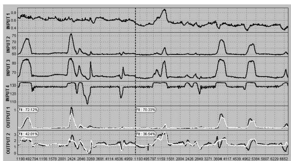
Figure 4: Model validation through simulation (simulated outputs in white)
