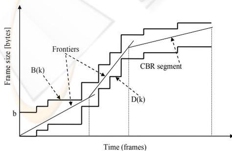
Figure 2a: An example of smoothed video stream transmission plan.
