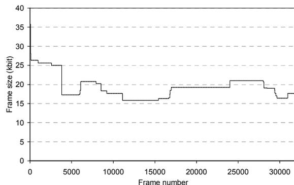
Figure 2b: The “Simpson’s” cartoon, MVBA smoothed (buffer size 1024 kbytes).
