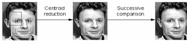
Figure 8: Centroid and Successive comparison reduction
