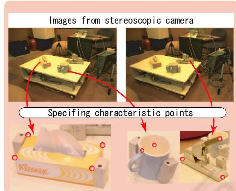
Figure 6: Photo-modeling by stereovision system
