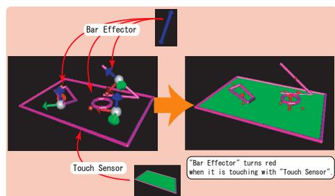
Figure 8: Create model of physical object's function using virtual sensors/effectors
