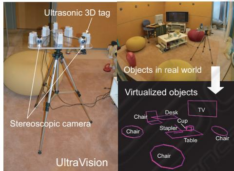
Figure 5: UltraVision for virtualizing objects and example of virtualized objects
