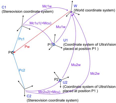
Figure 4: Coordinate Conversion in UltraVision system
