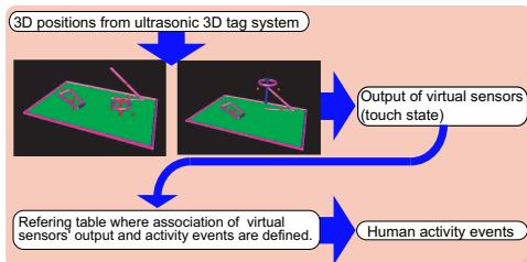
Figure 10: Real time detection and recognition of human activity by virtual object sensor
