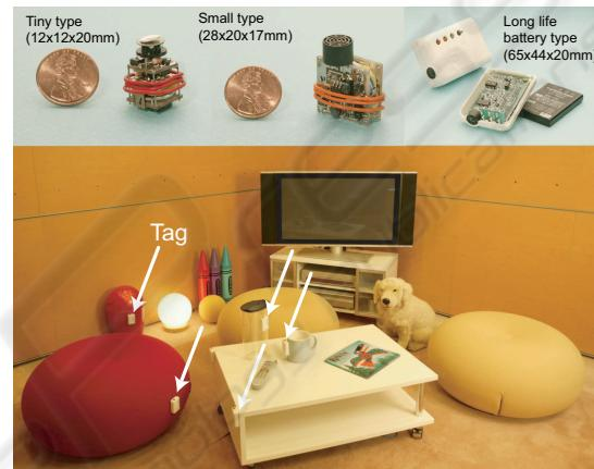
Figure 1: Ultrasonic 3D tag and sensorized environment
