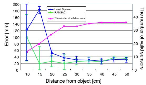
Figure 2: Accuracy of the ultrasonic tagging system when occlusion due to a hand occurs
