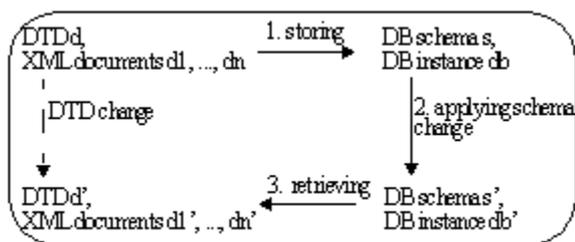
Figure 1: F2/XML method to manage DTD evolution
