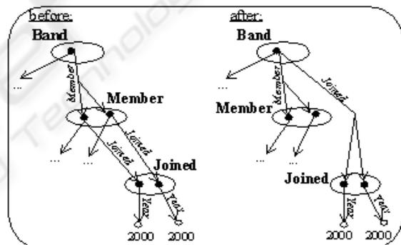
Figure 10: Updated database after changing the parent in the Member-Joined relationship to Band
