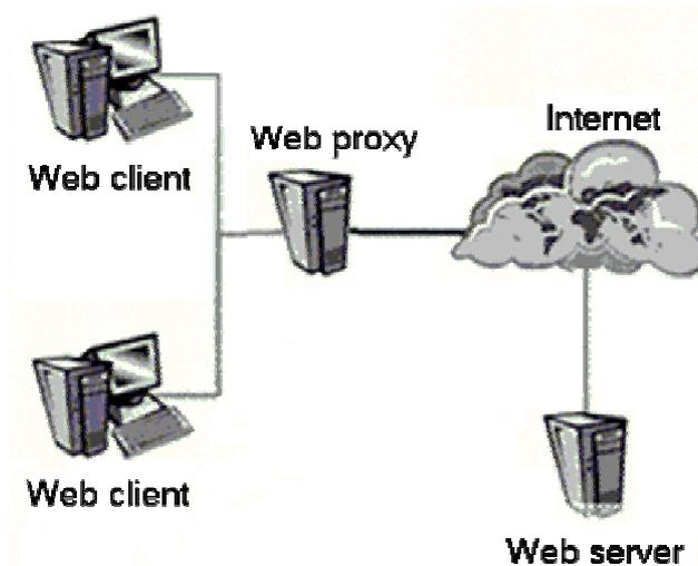
Figure 1: Web proxy in network configuration.
