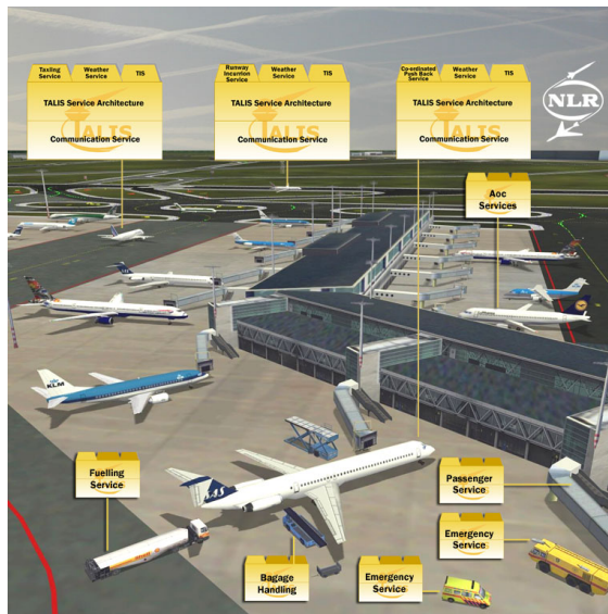
Fig. 2. Conceptual overview of the TALIS network-centric architecture
