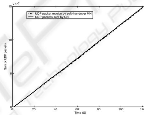
Figure 9. UDP received packets in Soft handover.
