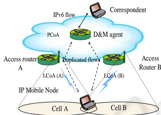
**Figure2:** IPv6 flow duplication and merging
