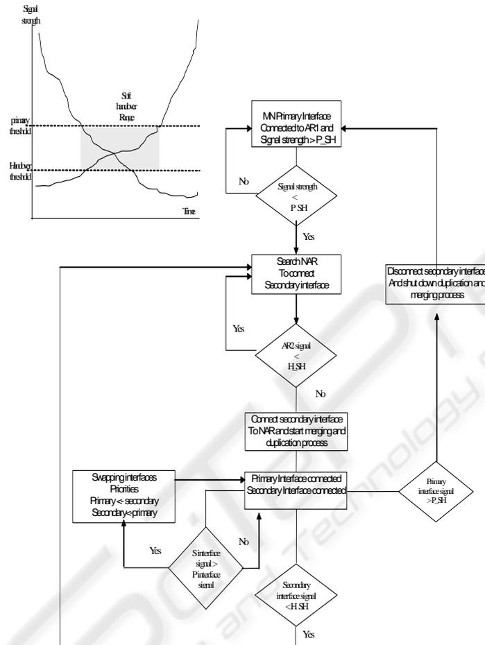
**Figure 4, 5:** Thresholds and Handover process
