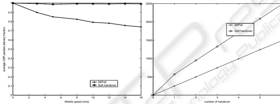
Figure 10. Average UDP packets fraction delivery
