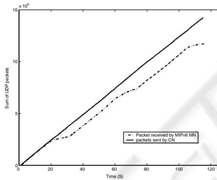
Figure 8 : UDP received packets in MIPv6.
