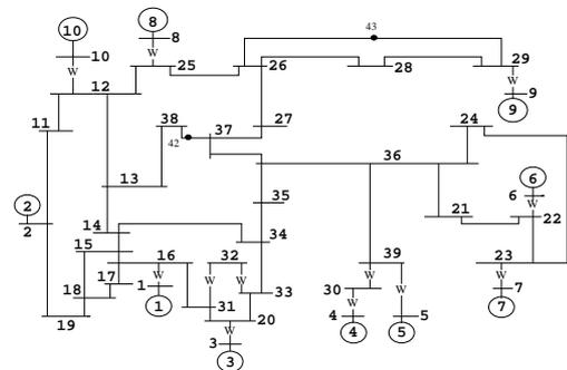
Figure 1: Single Line Diagram of 10 Machine 39-Bus System
