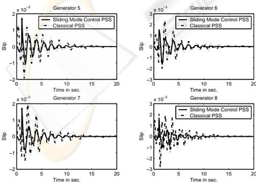
Figure 6: Nonlinear Simulation ( Slip)
