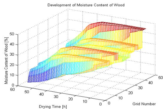
Figure 5: Evolution of the moisture content in the whole dried lumber for different values of the initial MC, and for each piece of wood
