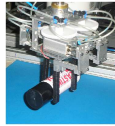
Figure 11: Developed gripper: configuration used to hold objects with cylindrical shape.
