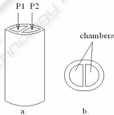
Figure 3: Physical structure of the tube
