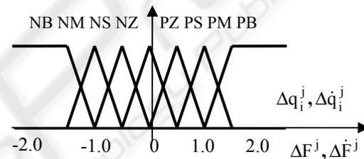
Figure 7: The membership functions for control variables
