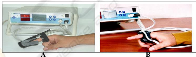
**Fig. 1.** Probe and monitor overview. **A** Fingertip probe **B** “Ring” probe
