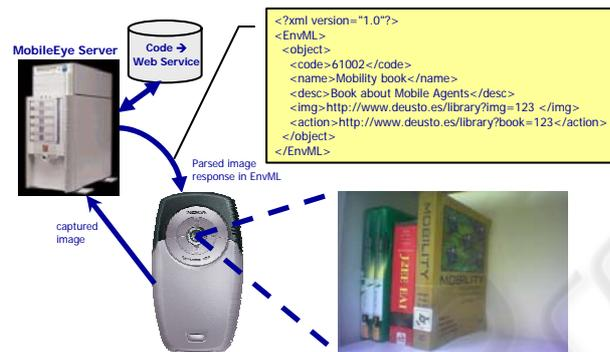
**Fig. 3.** MobileEye application architecture.
