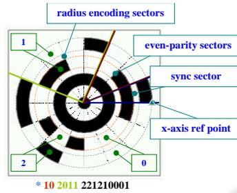
**Fig. 1.** TRIPcode of radius 58mm and ID 18,795. TRIP's 2-D printable and resizable ringcodes (*TRIPtags*) encode a ternary number in the range  $1-19,683(3^9 - 1)$  in the two concentric rings surrounding the bull's-eye of a target. These two rings are divided into 16 sectors.
