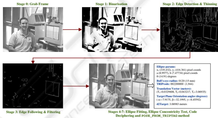
**Fig. 2.** Identifying and Locating the TRIPtag attached to a user's shirt in a 768x576 pixel image. Location extraction is only possible when the camera used is calibrated.
