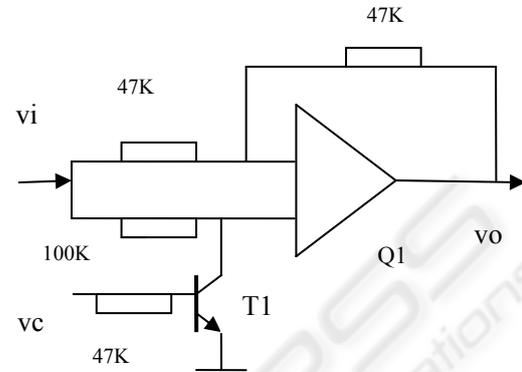
Figure 7: Controlled inverter circuit.
