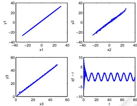
Figure 6: Synchronization between the hyperchaotic driver and response Lorenz systems with delay and variable parameters and the parameter  $q_1(t)$  of the response system as it identifies the driver signal  $p_1(t)$ .
