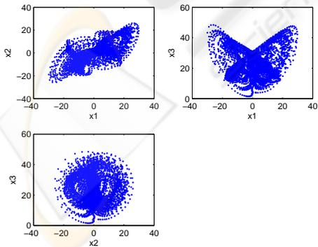
Figure 5: The hyperchaotic attractor of the driver Lorenz system with delay and variable parameter. The response system has a similar attractor.
