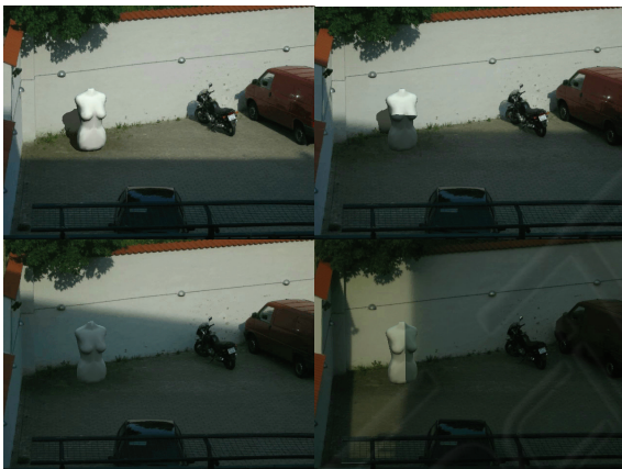
Figure 8: A scene displaying the systems ability to interact with the shadows of the environment. Furthermore it shows the ability to adapt the lighting to correspond to the surroundings, as well as displaying the necessity for a global illumination approximation for the ambient part of the shading, when the object is positioned in shadow.
