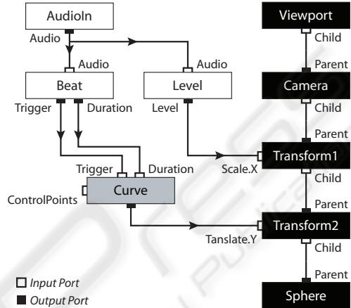
Figure 3: Simple processing graph example which represents an animated sphere driven by audio. White colored nodes depict the audio signal flow and black nodes represent the 3D scene graph. Additionally, an animation curve node is illustrated in grey.
