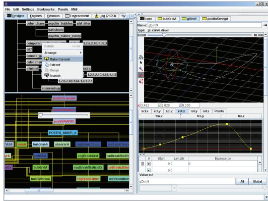
Figure 4: Screenshot of the graphical management console. Top left: Design tree which permits high-level editing. Bottom left: Processing graph representing the current system state. Right: Node inspector for modification of a selected processing node.
