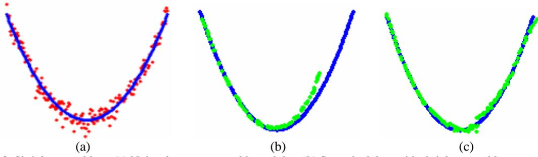
Figure 3: Shrinkage problem. (a) Noisy data represented by red dots (b) Smoothed data with shrinkage problem, represented by green dots (c) Smoothed data with shrinkage prevention using (8).
