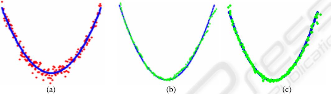
Figure 4: Bias correction (a) Noisy data represented by red dots (b) Smoothed data with bias problem, represented by green dots (c) Smoothed data with bias reduction prevention using (10).
