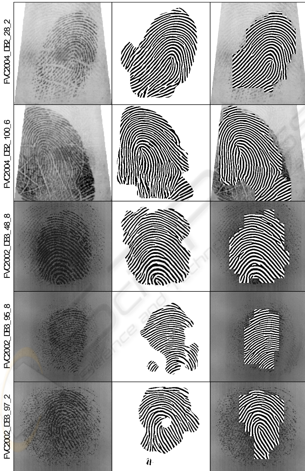
Figure 6: Comparison of segmentation between Neuro and the proposed. Left column is the original images; Middle column is the results by Neuro; Right column is the results by the proposed. The images in left column, from top to bottom, are respectively denoted as image4, image5, image6, image7 and image8.
