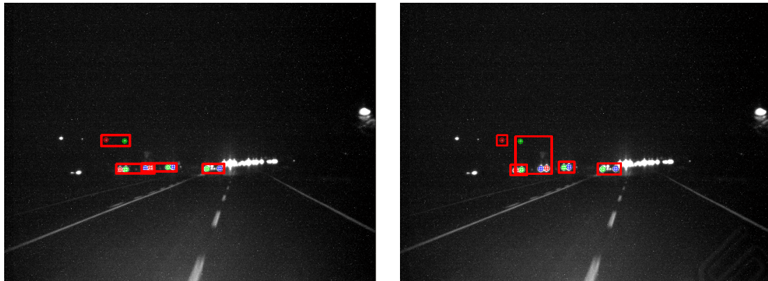
Figure 5: Sequence 1: four cars (three approaching the camera, one in the same direction) and two lamp posts. Left: Costeira–Kanade method, the three cars of the left are considered a unique object. Right: Han–Kanade method, one lamp post is grouped with one of the cars.
