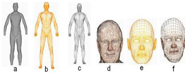
Figure 5: 3D-3D conformation technique: the 3D model (b) is fitted to the scan data (a), the result (c) is a human body model that embeds the shape of the scanned human body. (d,e and f) the same technique applied for the case of a human head.
