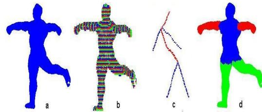
Figure 3: Segmentation of HB scan data for an arbitrary posture (a). Computation of the Level-sets (sets of data points located at the same geodesic distance with respect to a source point)(b). Construction of the Discrete-Reeb Graph (c) (a graph that encompasses the human body template, and which is invariant to posture changes). The segments and the joints of the graph are then mapped to the scan data to extract the different body parts (d).
