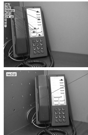
Figure 1: Specification of the virtual labels in reference image 1 (top) and guided insertion (i.e. the associated point must be on the epipolar line shown) of 'redial' label in the second reference image (bottom).
