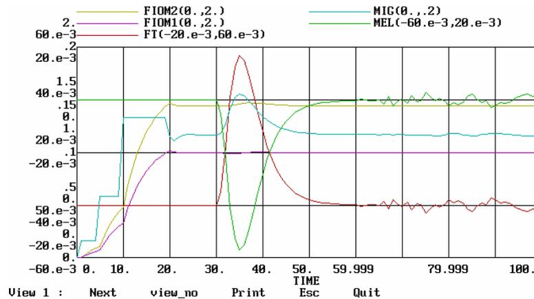
**Fig. 3.** Relative angular speed variation, relative angular speed variation of second shaft, generator electromagnetic moment, relative variation of fuel consumption.
