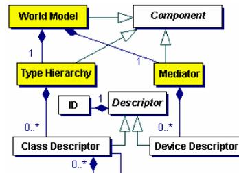
Figure 7: Model Components and Descriptors.
