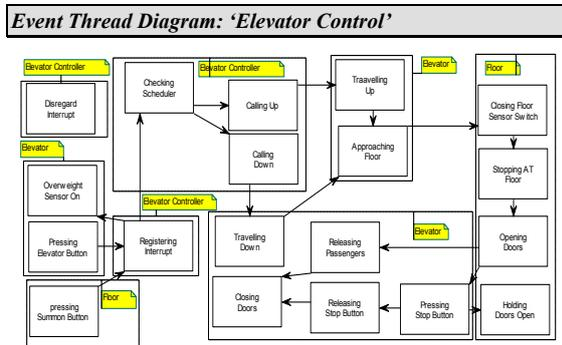
Figure 4: Event Thread –Elevator Control System.
