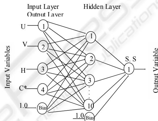
Figure 1: Typical three layers Feed-Forward ANN.
