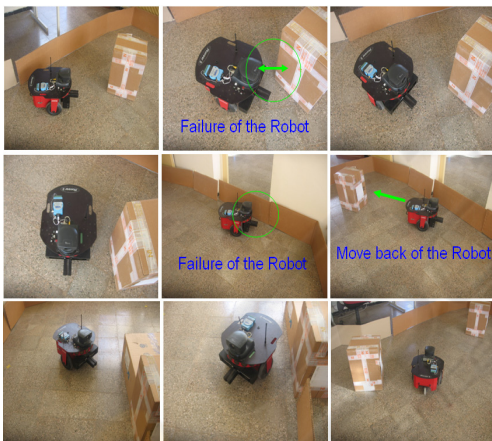
Figure 13: On line learning of the real robot Pioneer II, behaviour "Obstacle Avoidance".
